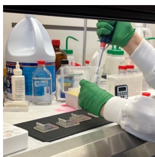
Photo 11: A scientist loading devices containing MDTs with a formalin solution for fixation
