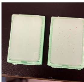
Photo 12: MDTs embedded in paraffin for preservation (visible as pink dots in the righthand bloc)
